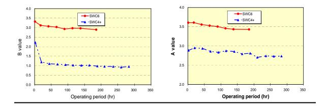
The SWC4+ Max elements are being tested at a pilot site also on the Pacific Ocean. This test is operating at 8.9 gfd flux, 21 to 23 C, and 51% recovery with 6 elements in the pressure vessel.
