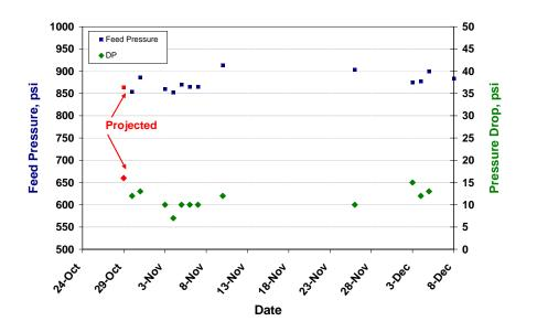
The results show that the performance of these new high area elements is very stable over the three month trial period. The projected feed pressure agrees quite well with the actual results, and the normalized pressure drop is actually lower than the actual value, 16 psi, versus 13 psi. Thus, it can be seen that the high area element performance is a logical extrapolation from the current, know membrane performance.
